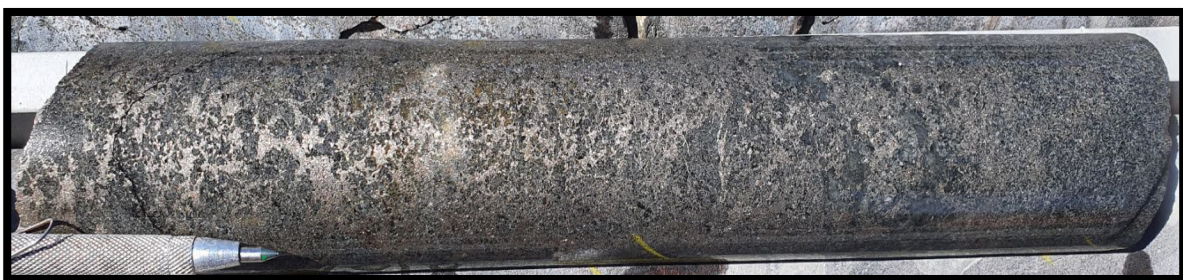
Photo 1: Net-textured and heavy disseminated Ni-Cu sulphide from RKDD033 from 394m, NQ2
